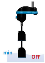
Low level stops the pump
